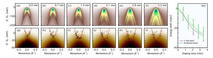
FIG. 2. (a)–(f) ARPES intensity plots of the hole band at the  $\Gamma$  point, recorded with 60 eV photons. The black lines are Lorentzian fit results of the MDCs in the [-200, -100] meV range. (g)–(l) ARPES intensity plots of the electron band at the M point. The red curve is a parabolic fit for the electron band dispersion. (m) Comparison of the  $\Gamma$  hole band shift derived from (a)–(f), and the electron band shift from (g)–(l).
