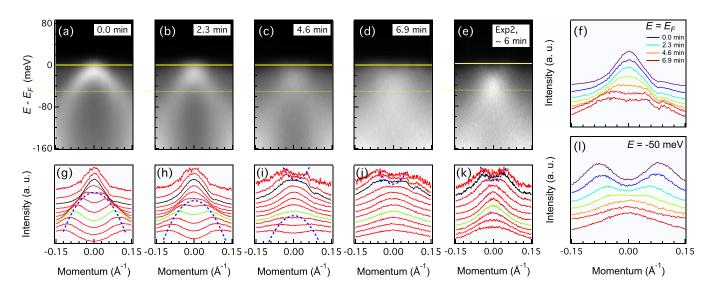
FIG. 3. (a)–(d) ARPES intensity plots around at  $\Gamma$  with doping time, recorded with 30 eV photons. (e) Similar experiment made with another sample. (g)–(k) Corresponding MDC plots. The MDCs in black refer to  $E_F$  while the ones in green have been measured 50 meV below  $E_F$ . The dashed lines are guides to the eye for the band dispersion. (f) MDCs at  $E_F$  with doping time. (l) MDCs 50 meV below  $E_F$  as a function of doping time.
